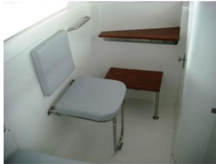
Collapsible seat for Crew near from exit
