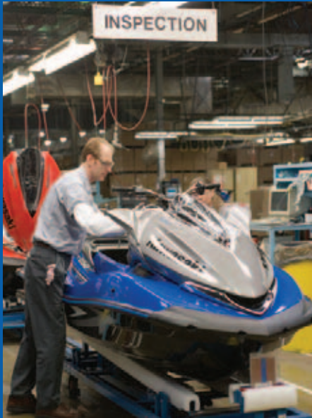
From left: Once the hull and deck are joined together, the new Ultra 250Xs receive finishing touches including the decals, rubrails and seats. Completed models are then sent to the quality control area where they are inspected for flaws before being packaged in wooden crates and shipped out to dealerships.
