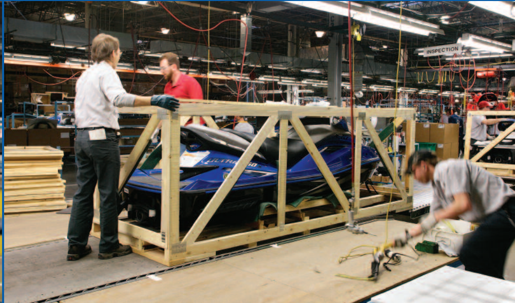
From left: Once the hull and deck are joined together, the new Ultra 250Xs receive finishing touches including the decals, rubrails and seats. Completed models are then sent to the quality control area where they are inspected for flaws before being packaged in wooden crates and shipped out to dealerships.
